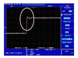
Probe Cable Bending
